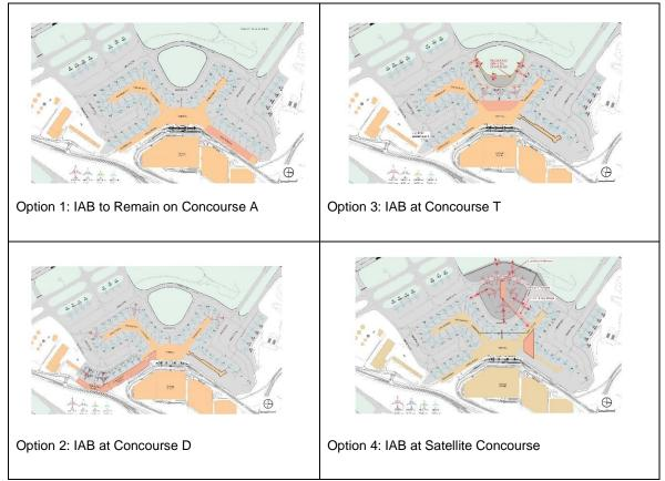
Figure 3.3-4: Initial Concepts for Permanent IAB
